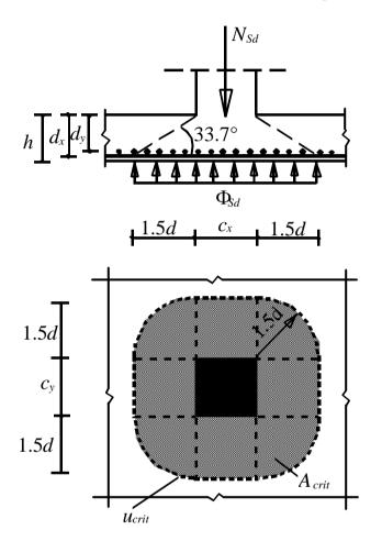
Figure 4 Critical section for punching shear according to EC 2
