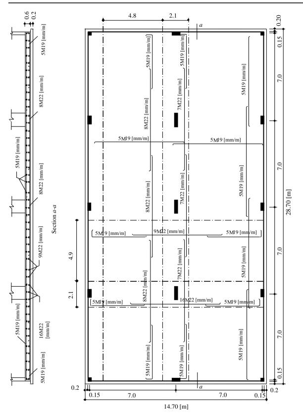
Figure 72 Details of reinforcement in plan and section *a-a* through the raft
