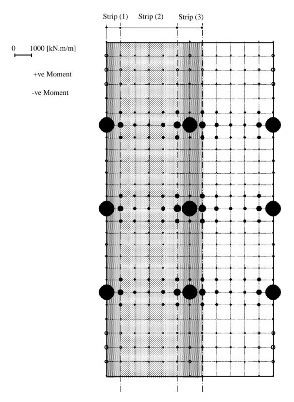
Figure 66 Circular diagrams of moments  $m_y$  [kN.m/m] and critical strips in y-direction
