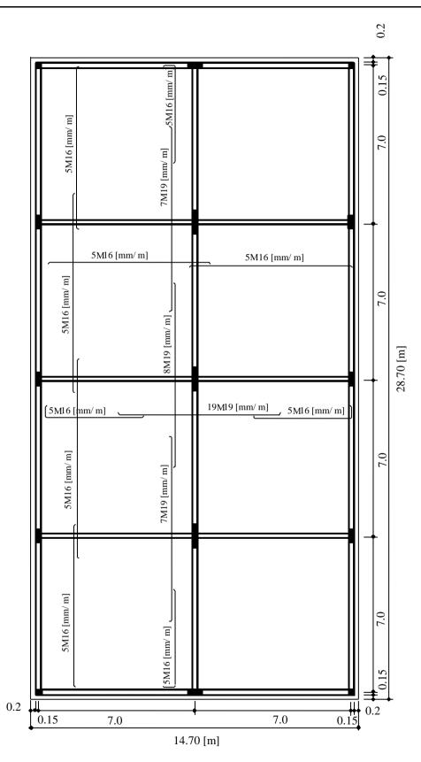
Figure 79 Details of reinforcement in plan
