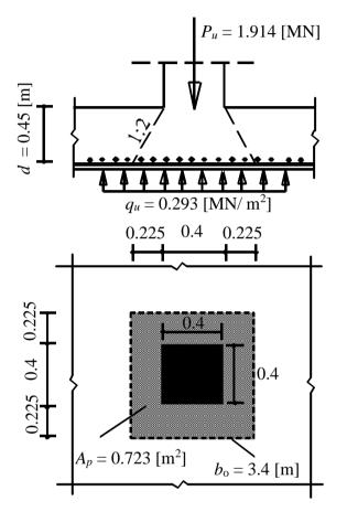
Figure 18 Critical section for punching shear according to ACI
