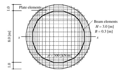
Figure 35 Rectangular finite element mesh
