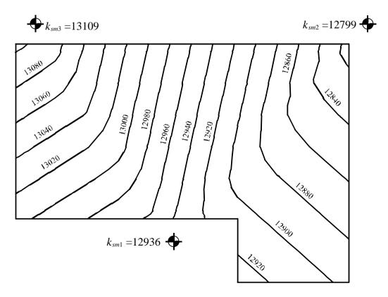
Figure 26 Contour lines for variable modulus of subgrade reaction  $k_s$  [kN/m<sup>3</sup>]
