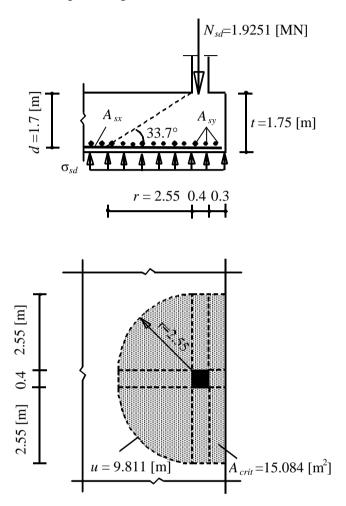
Figure 31 Critical section for punching shear according to EC 2
