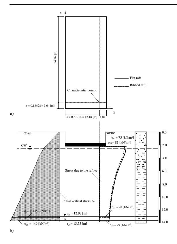
Figure 60 a) Position of characteristic point cb) Limit depth  $t_s$  of the soil under the rafts
