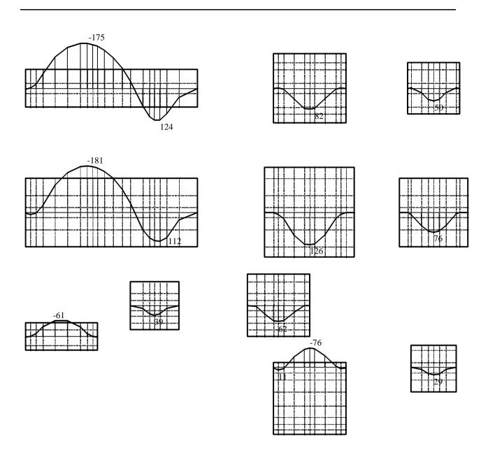
Figure 90 Moment  $m_x$  [kN.m/m] at critical sections on the footings
