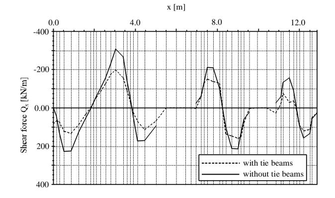
Figure 102 Shearing force  $Q_x$  [kN/m] at section 2-2
