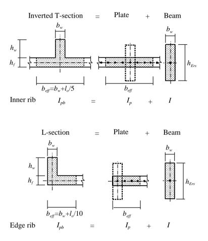
Figure 52 Determination of replacement height  $h_{Ers}$
