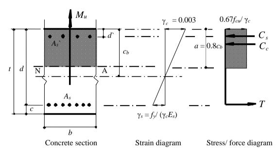
Figure 9 Distribution of stresses and forces according to ECP (limit state method)
