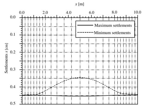
Figure 38 Extreme values of settlements *s* [cm] in *x*-direction under the raft with effect of the wall
