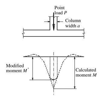
Figure 71 Modified moment under the column
