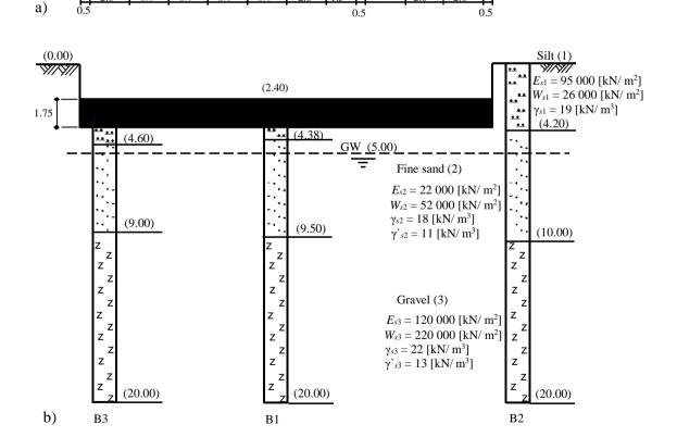
Figure 24 a) Plan of the raft with column loads, dimensions and mesh b) Section through the raft and subsoil
