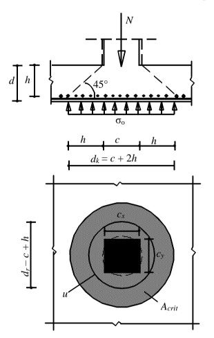
Figure 6 Critical section for punching shear according to DIN 1045
