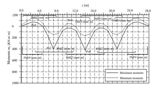
Figure 70 Extreme values of moments  $m_y$  [kN.m/ m] in field strip (2)
