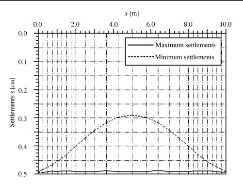
Figure 37 Extreme values of settlements *s* [cm] in *x*-direction under the raft without effect of the wall
