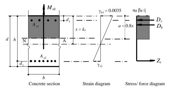
Figure 5 Distribution of stresses and forces according to DIN 1045
