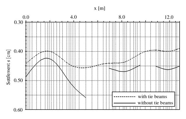
Figure 100 Settlement *s* [cm] at section 2-2
