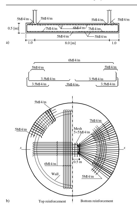
Figure 48a) Section x-x through the raft with reinforcementb) Reinforcement of the raft in plan
