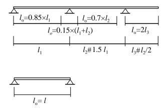
Figure 53 Definition of effective span  $l_0$
