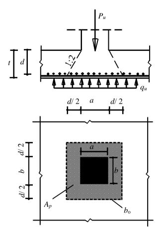
Figure 10 Critical section for punching shear according to ECP (limit state method)
