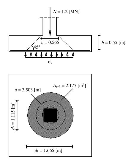
Figure 23 Critical section for punching shear according to DIN 1045
