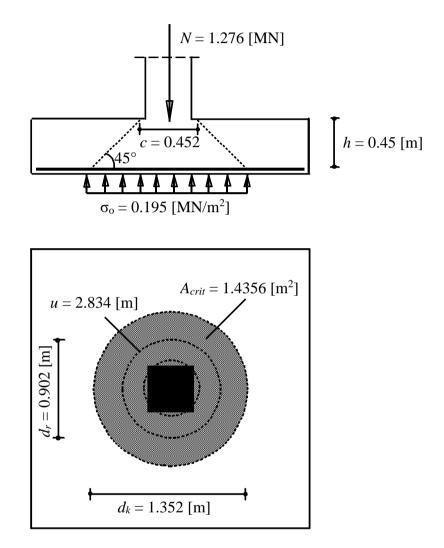
Figure 17 Critical section for punching shear according to DIN 1045
