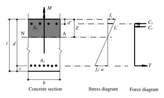
Figure 11 Distribution of stresses and forces according to ECP (working stress method)
