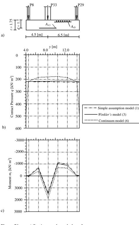
Figure 29 a) Section *y*-*y* through the raft
