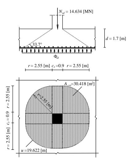
Figure 30 Critical section for punching shear according to EC 2
