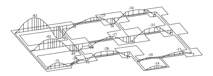
Figure 97 Moment  $M_b$  [kN.m] in girders at longitudinal and diagonal directions
