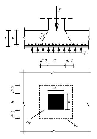
Figure 12 Critical section for punching shear according to ECP (working stress method)
