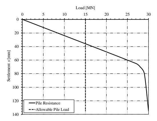
Figure 8-5 Load-settlement relation from pile load test
