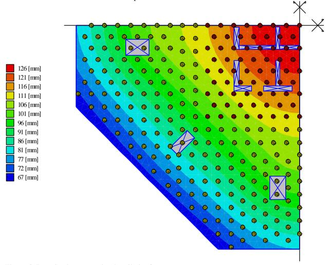
Figure 8-7 Settlement under the piled raft
