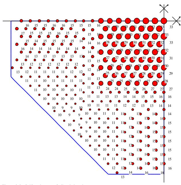
Figure 8-8 Self settlement of piles  $S_{\nu}$  [mm]
