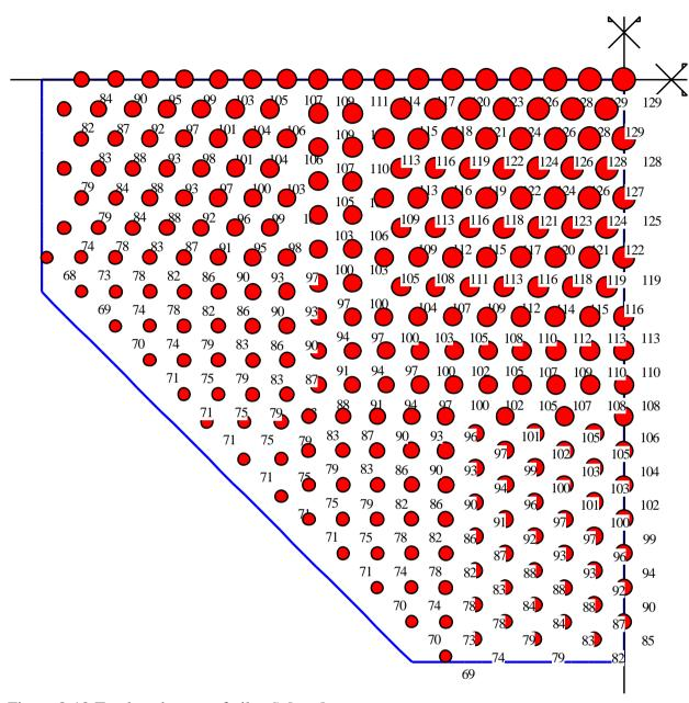
Figure 8-10 Total settlement of piles  $S_r$  [mm]
