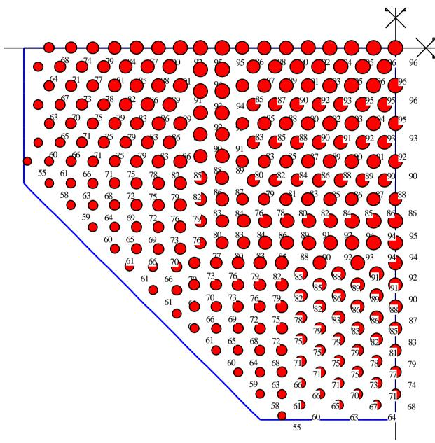
Figure 8-9 Interaction settlement of piles  $S_{rv}$  [mm]
