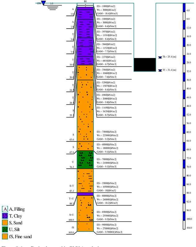
Figure 8-6 Boring log used in *ELPLA* analysis
