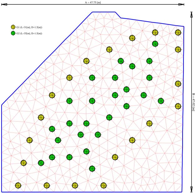
Figure 6-3 Mesh of *Skyper* piled raft with piles
