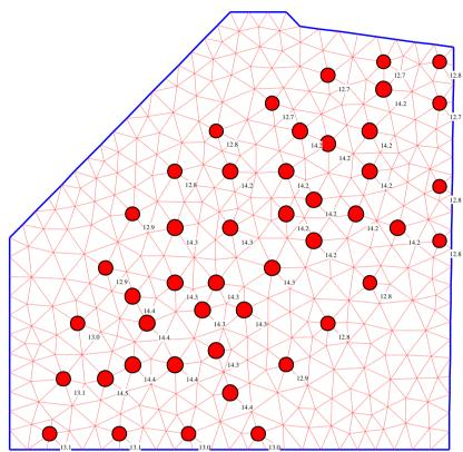
Figure 6-7 Pile load [MN] for rigid piled raft using German recommendations EA-Piles for upper values
