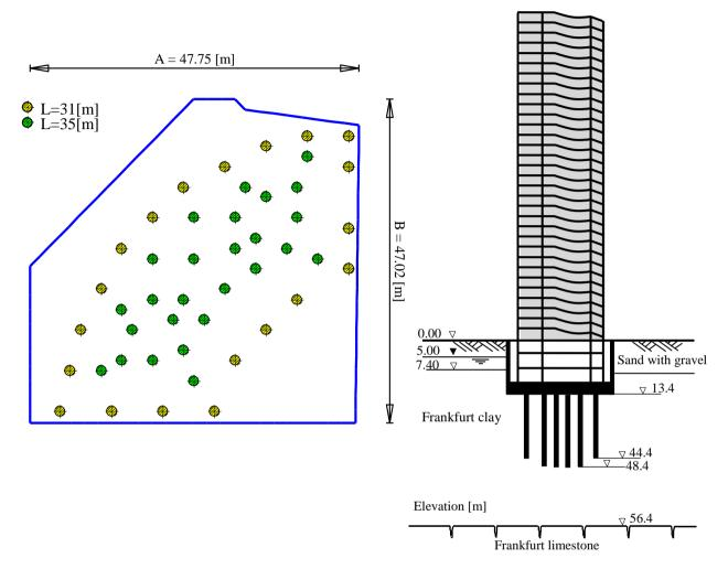
Figure 6-2 shows a layout of the *Skyper* piled raft foundation.
