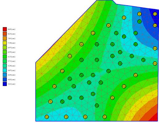
Figure 6-6 Settlement for elastic piled raft using German recommendations EA-Piles for upper values
