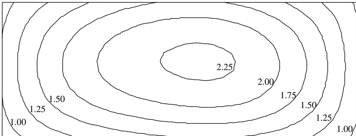
**Figure 4.42** Contour lines of settlements  $s$  [cm]
