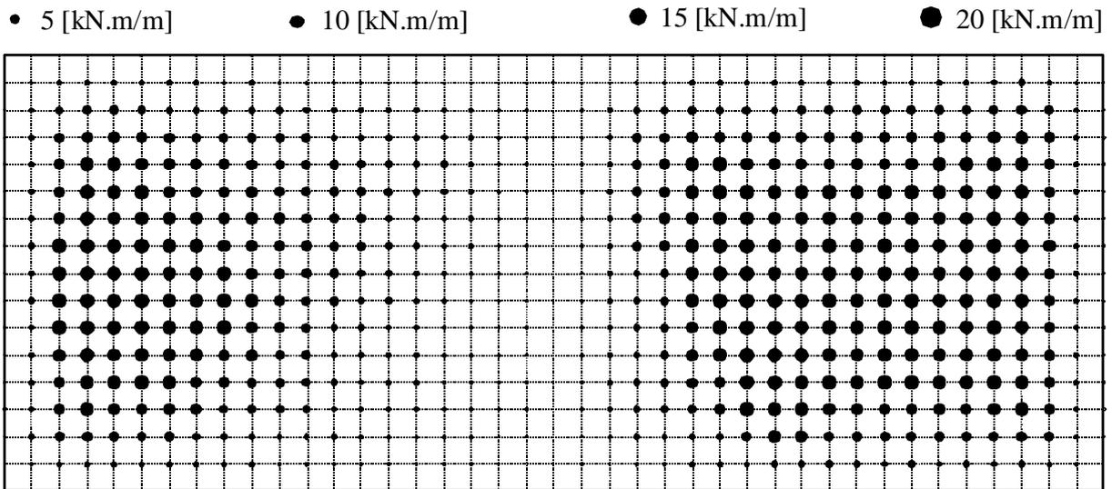
Figure 4.49 Circular diagrams of moments  $m_x$  [kN.m/m]
