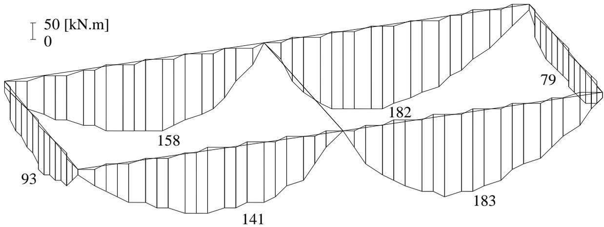
**Figure 4.52** Beam-bending moments  $M_b$  [kN.m] at edge walls of the swimming pool
