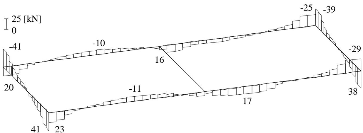
**Figure 4.57** Beam-Shearing forces  $Q_s$  [kN] at edge walls of the swimming pool
