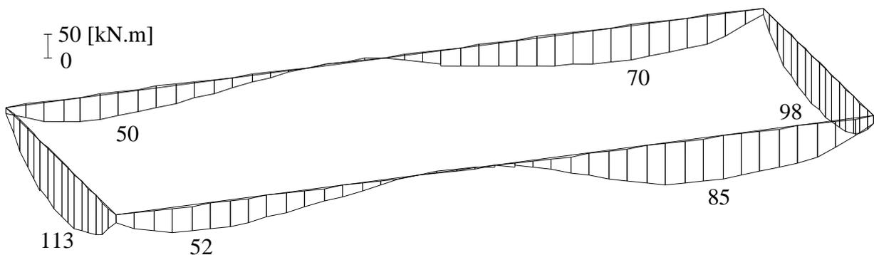
**Figure 4.54** Beam-bending moments  $M_b$  [kN.m] at edge walls of the swimming pool
