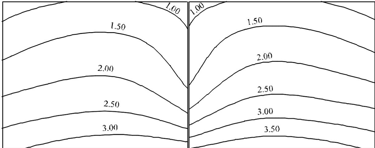
Figure 4.61 Contour lines of settlements  $s$  [cm]
