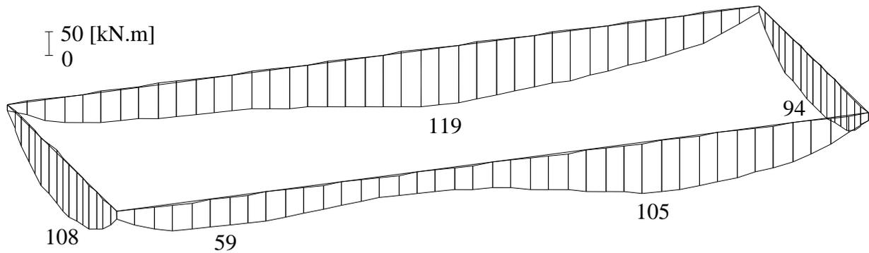
**Figure 4.55** Beam-bending moments  $M_b$  [kN.m] at edge walls of the swimming pool
