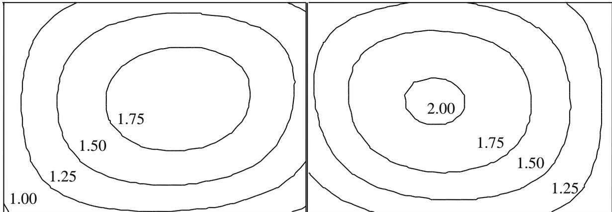
**Figure 4.39** Contour lines of settlements  $s$  [cm]
