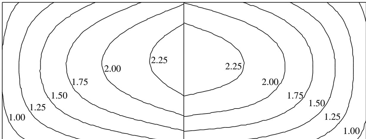
**Figure 4.40** Contour lines of settlements  $s$  [cm]
