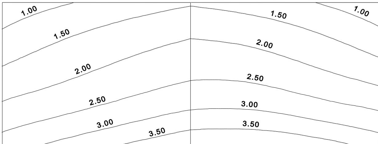
Figure 4.62 Contour lines of settlements  $s$  [cm]
