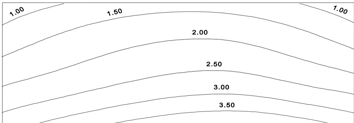
**Figure 4.64** Contour lines of settlements  $s$  [cm]
