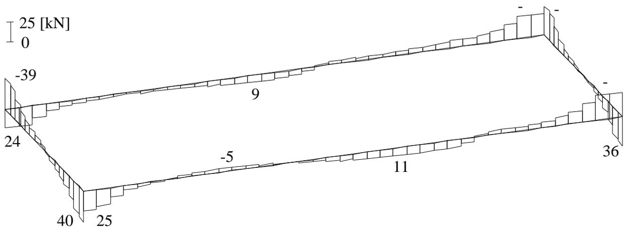
**Figure 4.59** Beam-Shearing forces  $Q_s$  [kN] at edge walls of the swimming pool
