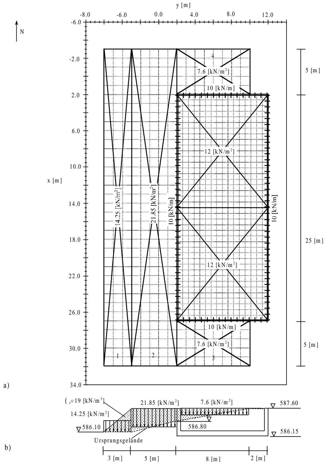
Figure 4.38 Swimming pool with loads and external loaded areas 1 to 4
