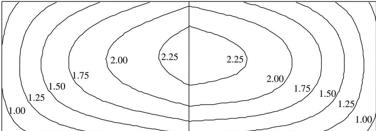
**Figure 4.41** Contour lines of settlements  $s$  [cm]
