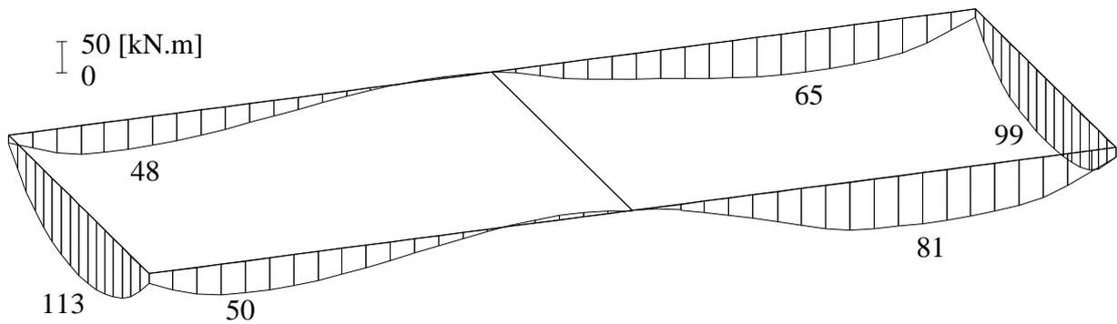
**Figure 4.53** Beam-bending moments  $M_b$  [kN.m] at edge walls of the swimming pool
