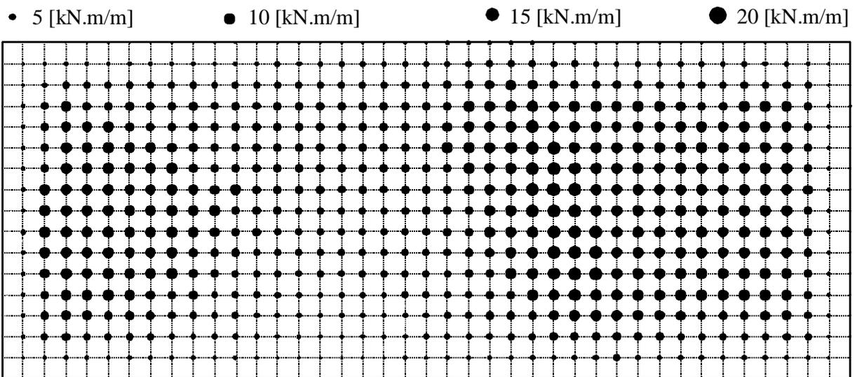
Figure 4.50 Circular diagrams of moments  $m_x$  [kN.m/m]
