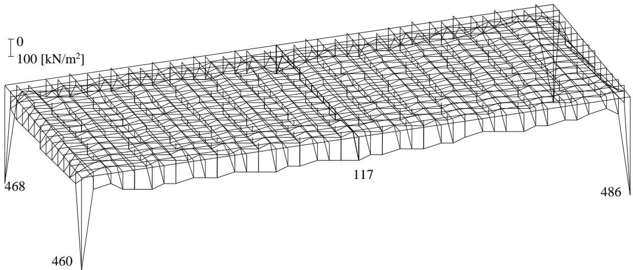
**Figure 4.45** Isometric view of contact pressures  $q$  [kN/m<sup>2</sup>]
