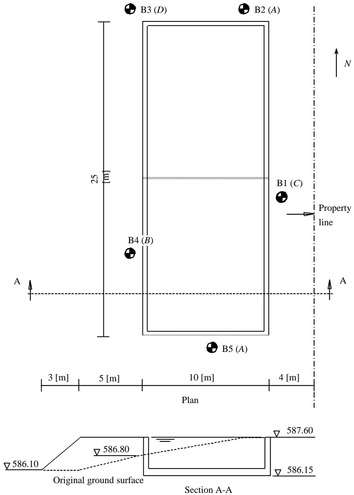
Figure 4.32 Details of the swimming pool
