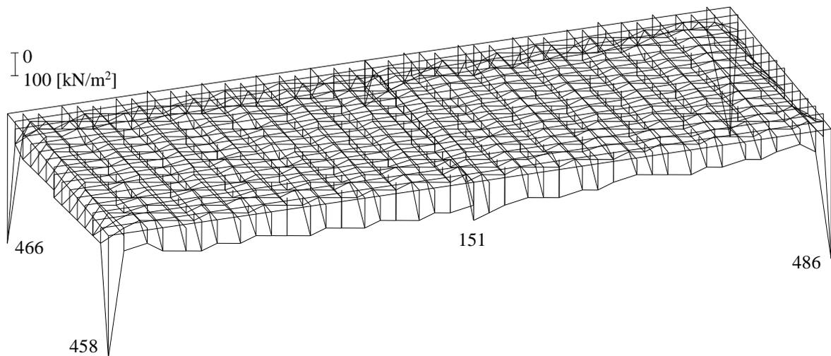
**Figure 4.44** Isometric view of contact pressures  $q$  [kN/m<sup>2</sup>]
