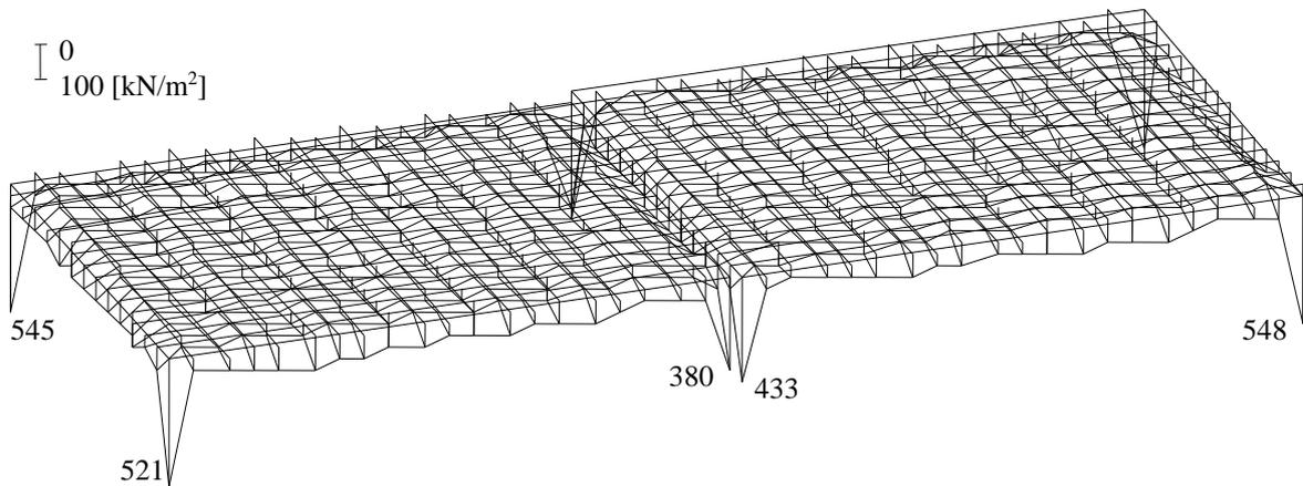
**Figure 4.43** Isometric view of contact pressures  $q$  [kN/m<sup>2</sup>]
