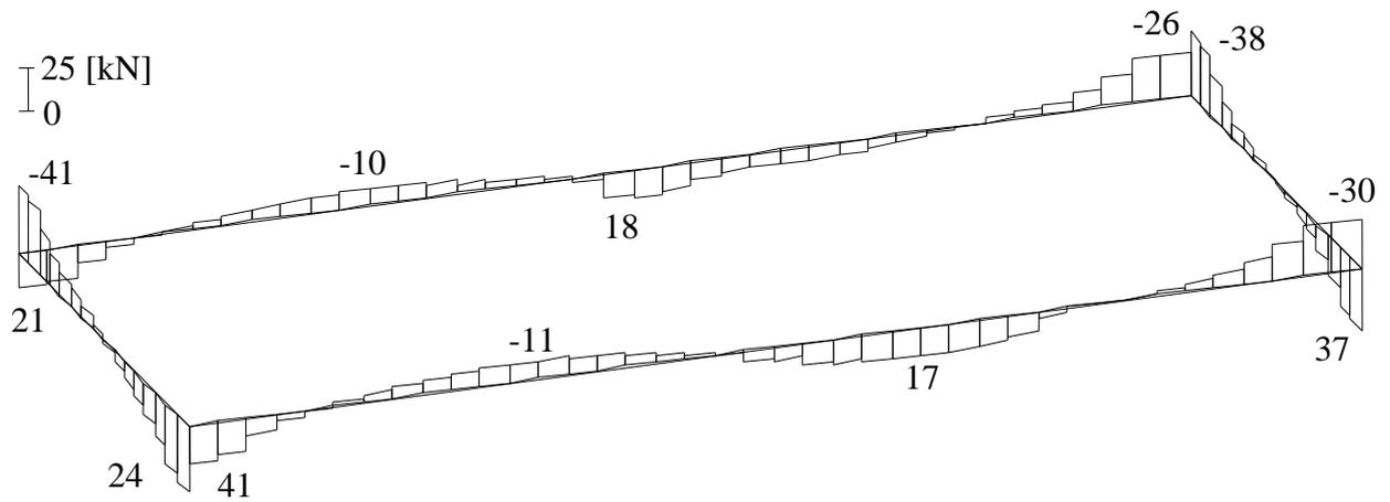
**Figure 4.58** Beam-Shearing forces  $Q_s$  [kN] at edge walls of the swimming pool
