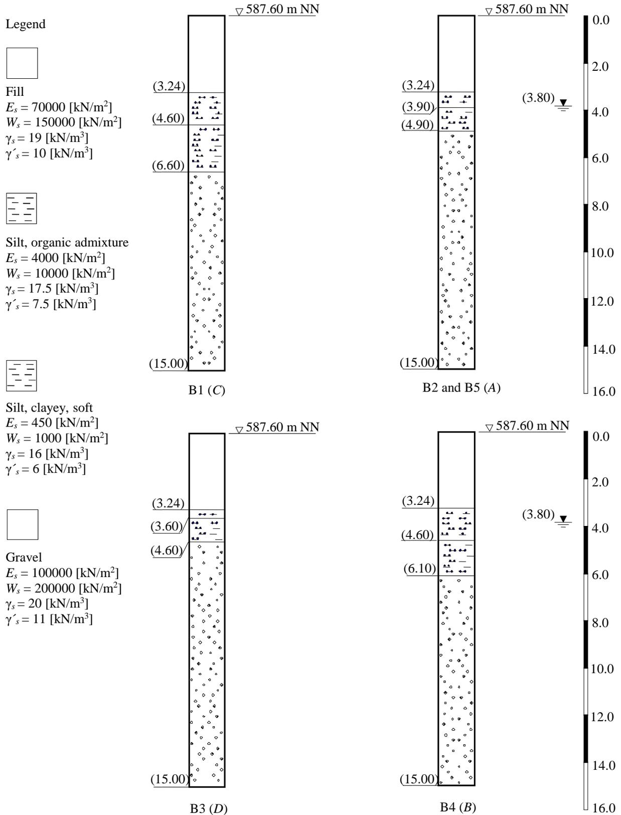
Figure 4.33 Boring logs B1 to B5 with soil properties
