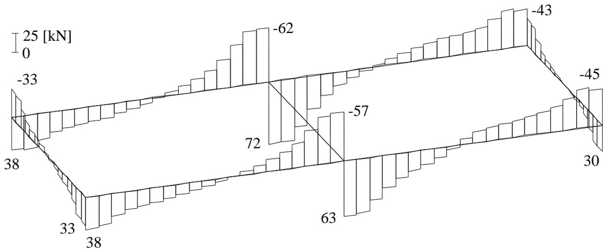
**Figure 4.56** Beam-Shearing forces  $Q_s$  [kN] at edge walls of the swimming pool
