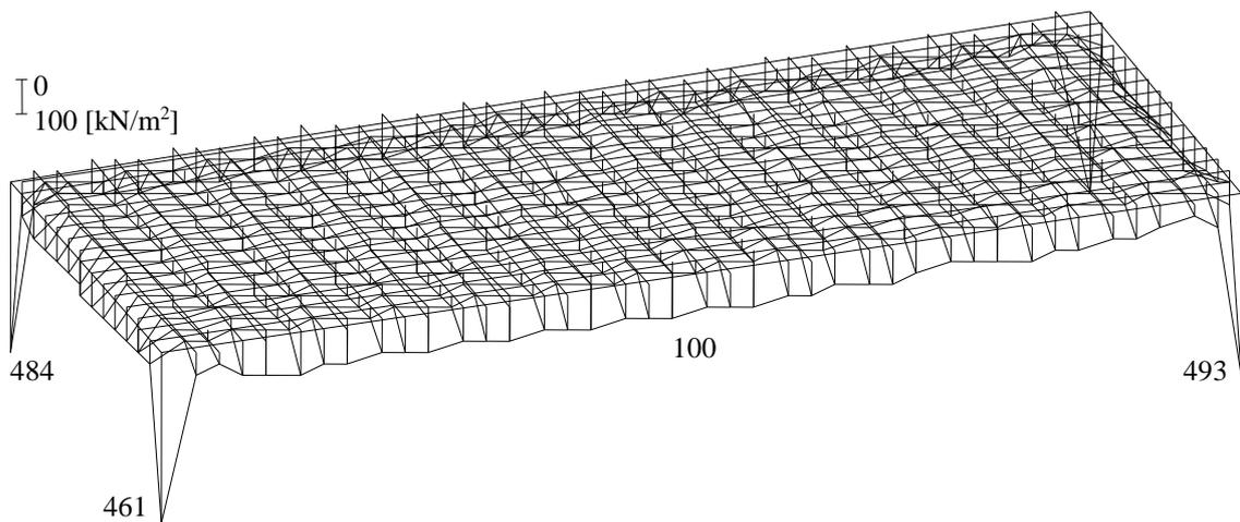
**Figure 4.46** Isometric view of contact pressures  $q$  [kN/m<sup>2</sup>]
