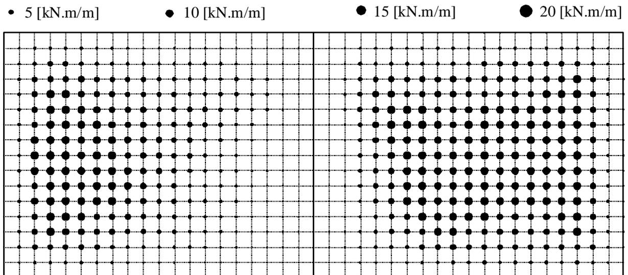
Figure 4.48    Circular diagrams of moments  $m_x$  [kN.m/m]
