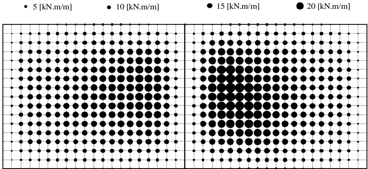
Figure 4.47    Circular diagrams of moments  $m_x$  [kN.m/m]
